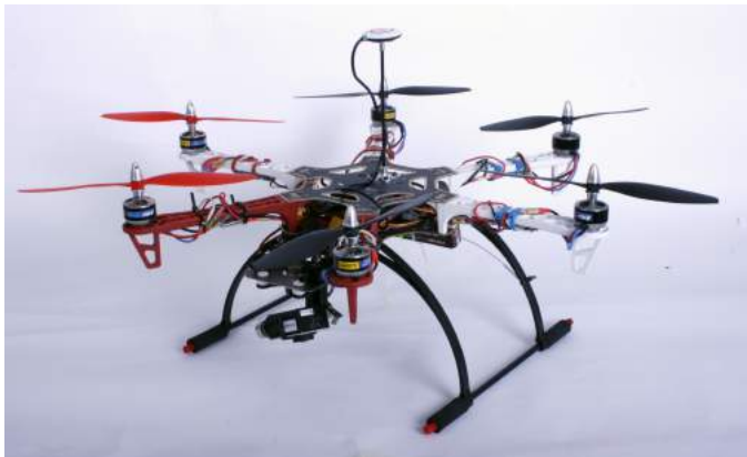
Fig. 2: One of the hexacopters used primarily for overland testing and filming. This hexacopter uses a DJI system that interfaces with a Lightbridge radio to stream HD video.
