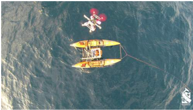
Fig. 9: Image from one of the fleet of SnotBots watching another SnotBot approach SnotShot , the whale surrogate. This was taken during field testing in the Gulf of Mexico Summer 2014.
